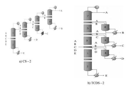
F~i~g~.~2~-~Sequence fully thermally coupled (TCDS-2) and the conventional sequence where~it~is~obtained
