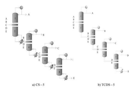
$Fig.\ 5\ - \textit{Sequence fully thermally coupled (TCDS-5) and the conventional sequence where it is obtained}$
