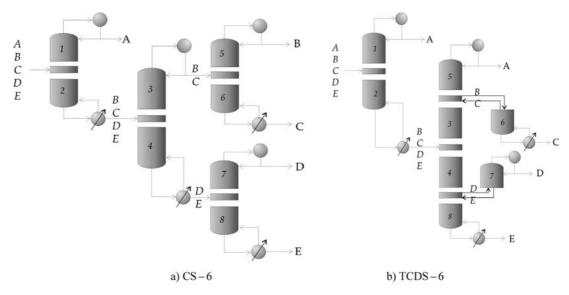
Fig. 6 - Sequence partially thermally coupled (TCDS - 6) and the conventional sequence where it is obtained
