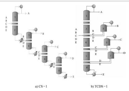
$Fig.\ 1\ -\ \textit{Sequence fully thermally coupled (TCDS-1) and the conventional sequence where it is obtained}$
