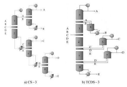
Fig. 3 – Sequence fully thermally coupled (TCDS – 3) and the conventional sequence where it is obtained
