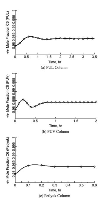
Fig. 7. Closed loop responses for a set point change in the composition of the intermediate component.
