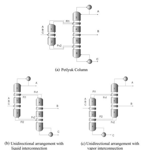
Fig. 4. Alternative schemes to the Petlyuk column.
