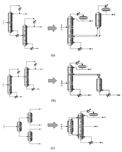
Fig. 3. Rearrangement of a conventional distillation sequence into the Petlyuk column.
