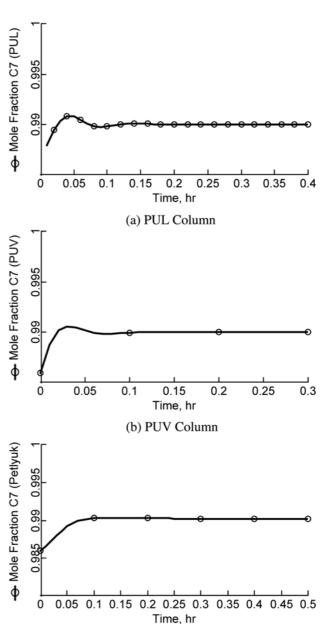
Fig. 5. Closed loop responses for a set point change in the composition of the heavy component.
