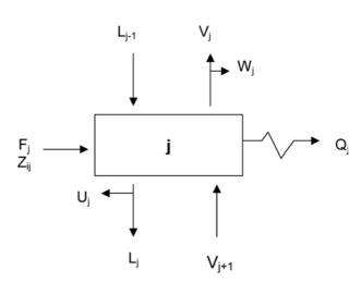
Fig. 2. A generic equilibrium stage for the model of the Petlyuk system.
